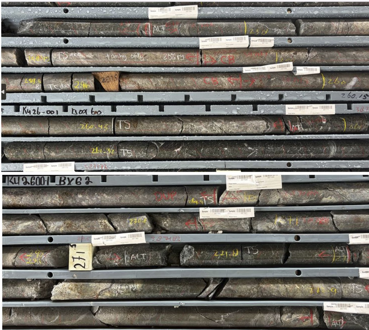
Image 2: KU26-01 intersected a strongly hydrothermally altered volcanic sequence characterized by abundant anhydrite and zones of significant disseminated to vein-hosted pyrite.
